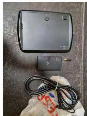
Relay theft device consisting of two units (large and small) and cable antennae
