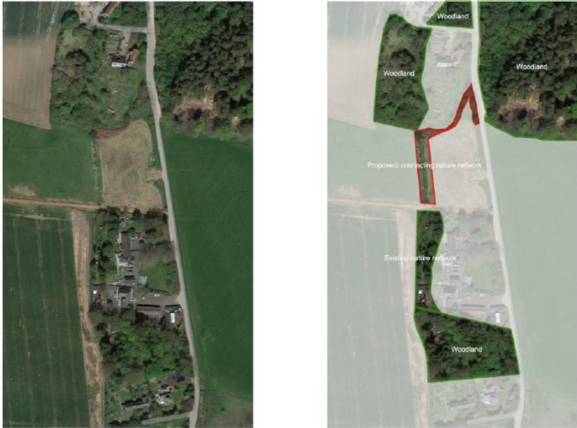
Figure 26 – Existing aerial to left with annotated aerial to right showing the existing nature network outlined in green and the proposed nature network in red that will link four woodland areas by following the existing watercourse.
