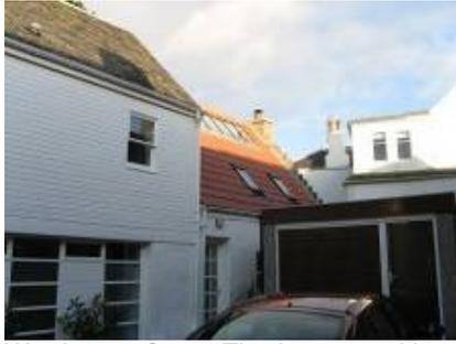
Warrington Court. The frontage with horizontal boarding is adjacent to listed no. 3 (harled, not in the photo) The house in the corner has a non-traditional door, concrete roof tiles with a large number of rooflights. The garage block clutters this small square.
