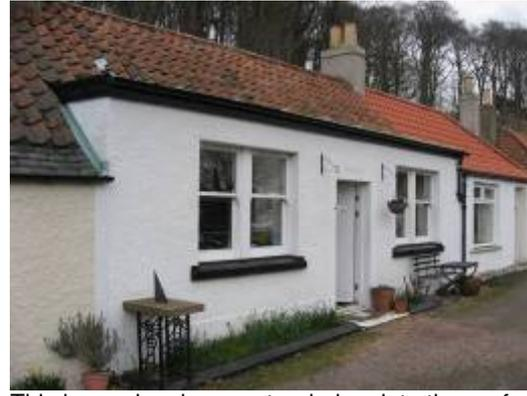
This house has been extended up into the roofspace and the window openings heightened.
